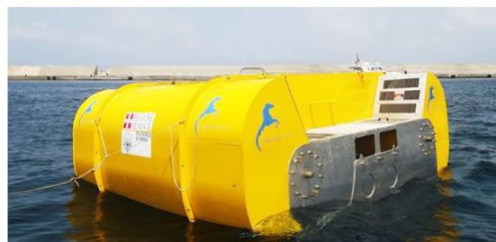
Figura 31 - ISWEC (Inertial Sea Wave Energy Converter)
